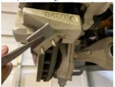
2. Once the clip is in place and secure, it may take a bit more than hand force to snap it into position.
