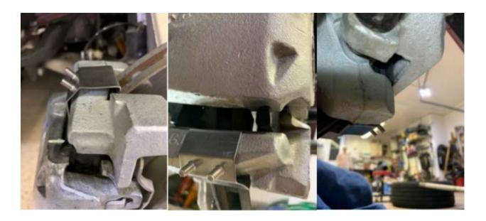
7. Once the clips are installed the caliper cover fits on as outlined in the instructions, no clearance issues between the clips and rotor.
